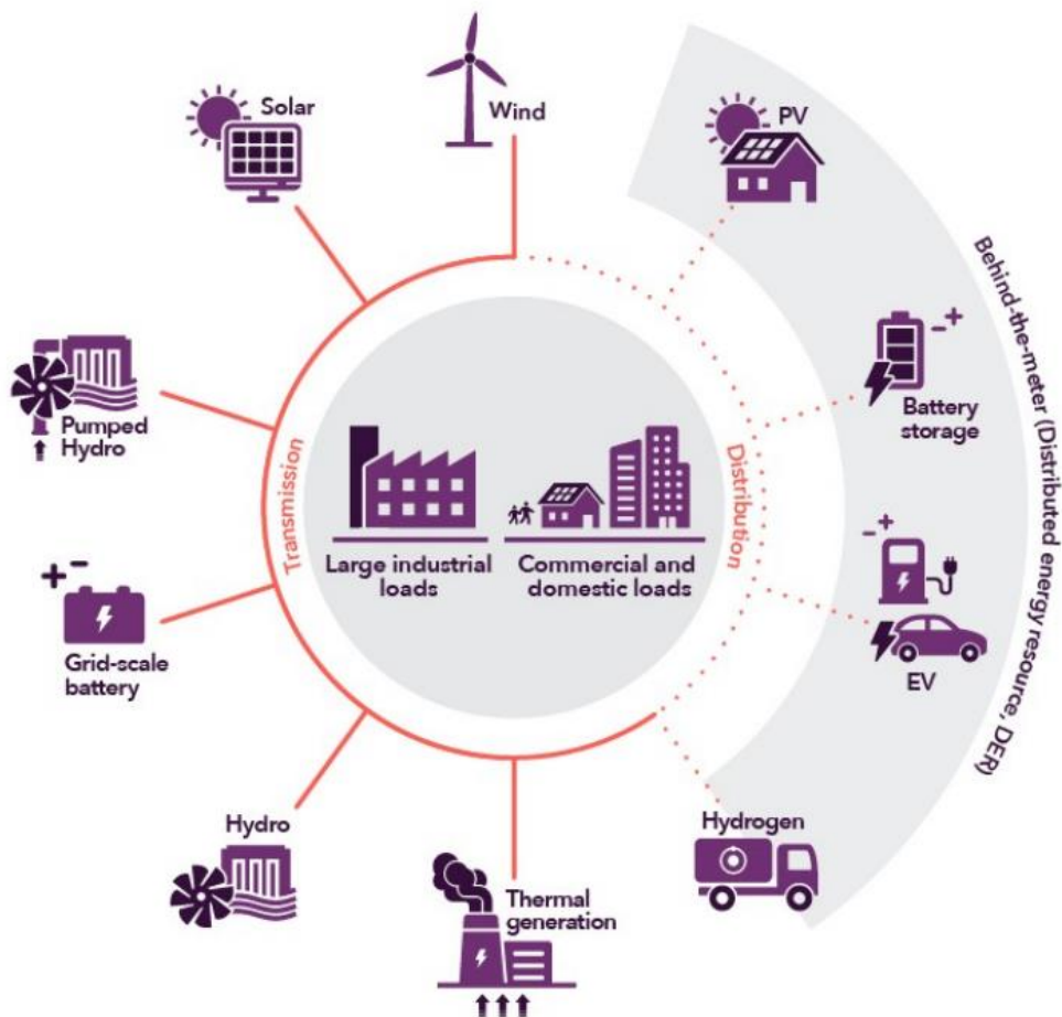
Figure 1 Power system interactions between grid and behind-the-meter energy supply (Figure 4 in ref [1])
