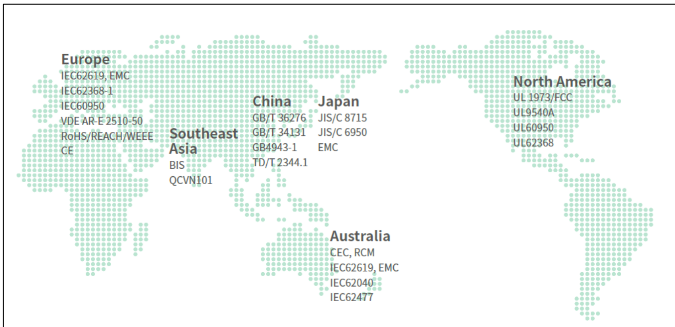
Figure 6 High level list of global standards used for BESS
